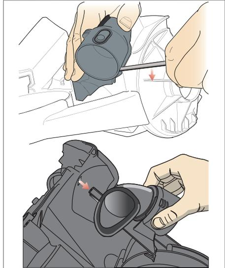
22 Then prise a thin, flat bladed screwdriver under the cyclone inlet and slide the inlet off the LMC assembly. To refit, slide onto the LMC assembly, refit the screw and neatly dress the loom within the ribs.
