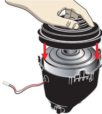
30 Fit the fan case seal onto the base of the motor.
